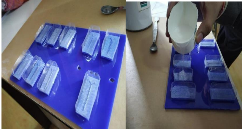
Fig. 7 Pouring of PDMS into Mold cavity
