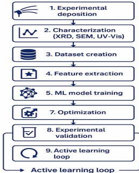
Figure2: Stepwise flow highlights how experimental data and machine learning interact to continuously refine synthesis conditions [18]
